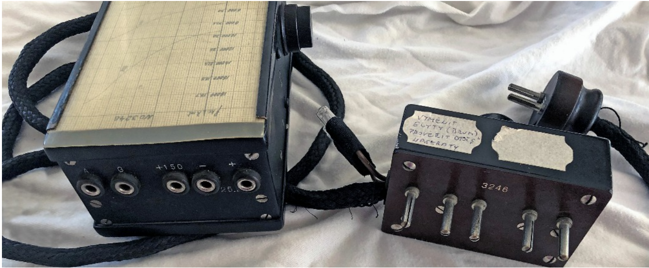
Right hand side view of the Signal 1 and separate power assembly with special mains cord and 12H6 rectifier valve.
